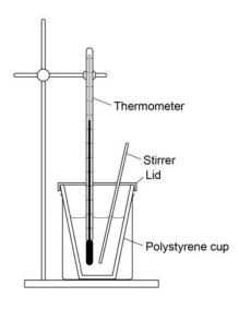
In an **enthalpy change** practical, the temperature change needs to be accurately measured. This is done by **minimising** heat loss or heat gain from the surroundings. A polystyrene cup and lid is used to **insulate** the reaction mixture from surroundings. The stirrer is used to ensure thermal energy is spread evenly in the reaction mixture. The bottom of the thermometer must be **in** the reaction mixture.
